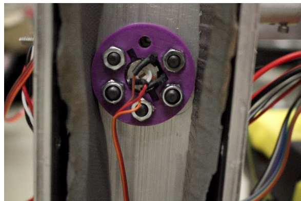
Figure 8. Potentiometer interfacing with C-Channel and pivot gearbox (behind C-Channel and not shown).
