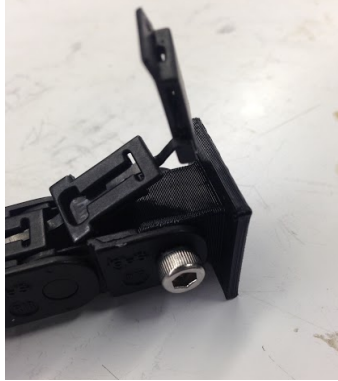
Figure 2. Test print of pin on cleaner that would interface with power chain
