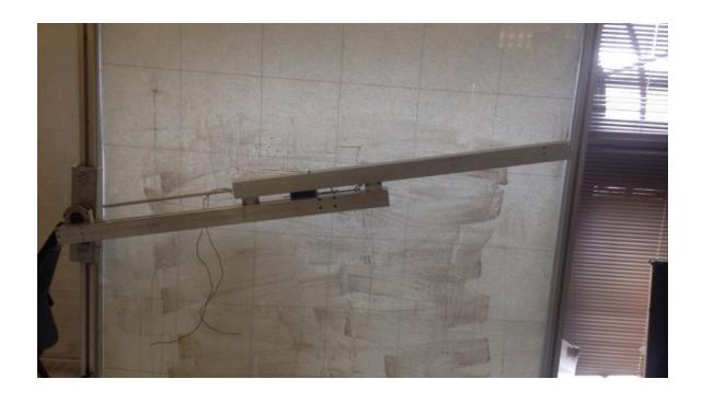
Figure 1 shows the robot hanging on the window using our passive gripper. This design uses the moment arm and weight of the robot to crate a friction hold on the window.
